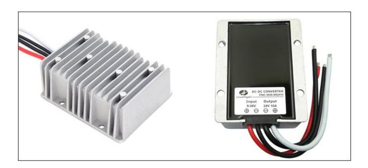
The WG9-36S2410 is a Non-isolated DC-DC converter that uses a synchronous rectification technology and features high efficiency and power density. It has the dimensions of  $100 \, \text{mm} \times 80 \, \text{mm} \times 39 \, \text{mm}$  and provides the rated output voltage of 24V and the maximum output current of  $10 \, \text{A}$ .
