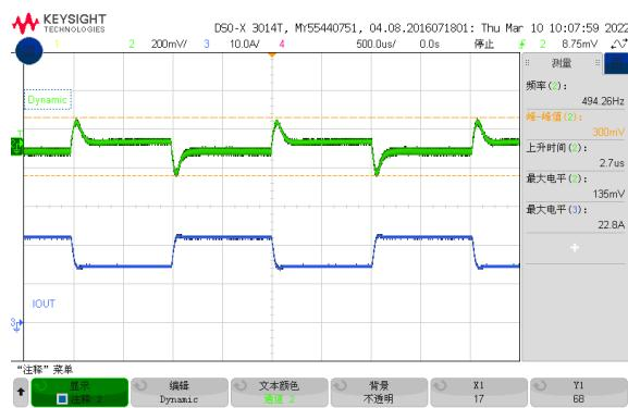
**Figure 6, Output voltage established (Iout = 30A)**
