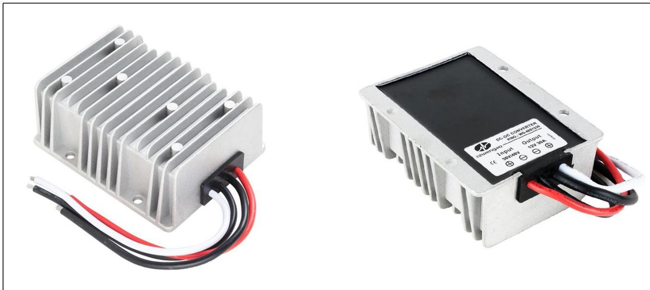
The WG-48S1230 is a Non-isolated DC-DC converter that uses a synchronous rectification technology, and features high efficiency and power density. It has the dimensions of 100mm x 80mm x 39mm (3.94 in. x 3.15 in. x 1.54 in) and provides the rated output voltage of 12V and the maximum output current of 30A.
