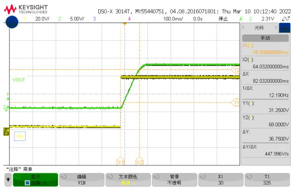
**Figure 9, Short-circuit & Output voltage (Iout = 30A)**
