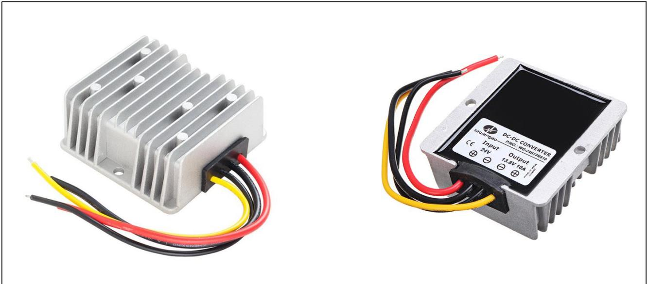
The WG-24S13R810 is a Non-isolated DC-DC converter that uses a synchronous rectification technology, and features high efficiency and power density. It has the dimensions of 74mm x 74mm x 32mm (2.91 in. x 2.91 in. x 1.26 in.) and provides the rated output voltage of 13.8V and the maximum output current of 10A.
