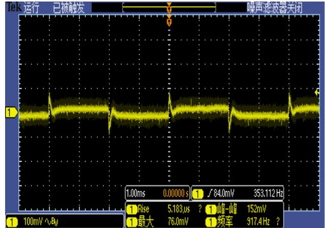
**Figure 6, Output voltage established (Iout = 10A)**
