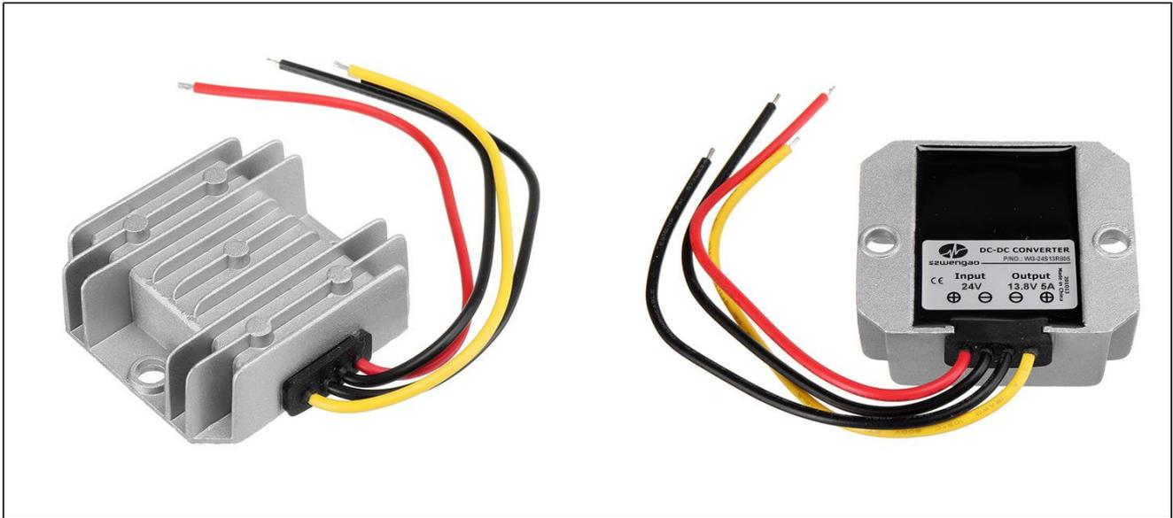
The WG-24S13R805 is a Non-isolated DC-DC converter that uses a synchronous rectification technology, and features high efficiency and power density. It has the dimensions of 64mm x 57mm x 22mm (2.52 in. x 2.24 in. x 0.87 in ) and provides the rated output voltage of 13.8V and the maximum output current of 5A.
