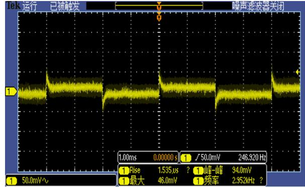
**Figure 6, Output voltage established (Iout = 5A)**
