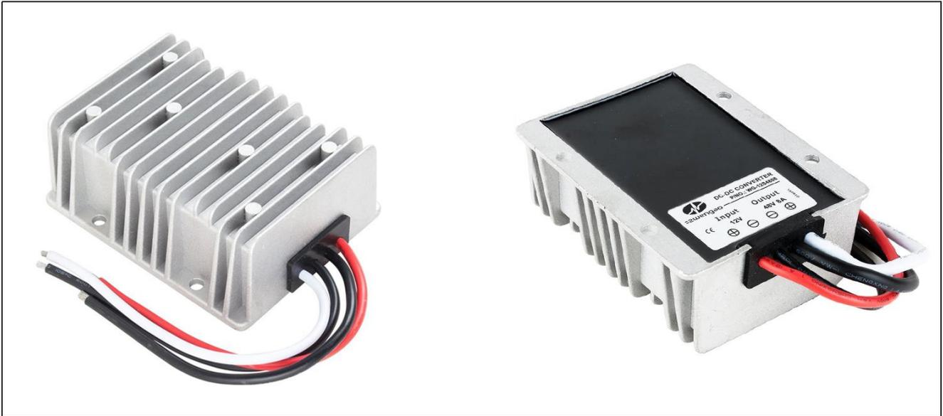
The WG-12S4808 is a Non-isolated DC-DC converter that uses a synchronous rectification technology, and features high efficiency and power density. It has the dimensions of 100mm x 80mm x 39mm (3.94 in. x 3.15 in. x 1.54 in) and provides the rated output voltage of 48V and the maximum output current of 8A.
