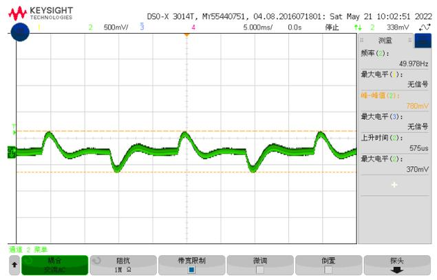
Figure 6, Output voltage established (Iout = 8A)
