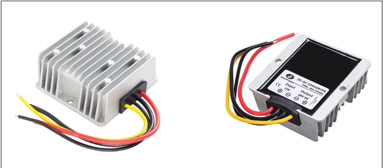
The WG-12S4805 is a Non-isolated DC-DC converter that uses a synchronous rectification technology, and features high efficiency and power density. It has the dimensions of 74mm x 74mm x 32mm (2.91 in. x 2.91 in. x 1.26 in) and provides the rated output voltage of 48 V and the maximum output current of 5A.
