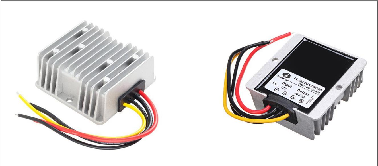
The WG-12S4803 is a Non-isolated DC-DC converter that uses a synchronous rectification technology, and features high efficiency and power density. It has the dimensions of 74mm x 74mm x 32mm (2.91 in. x 2.91 in. x 1.26 in) and provides the rated output voltage of 48V and the maximum output current of 3A.
