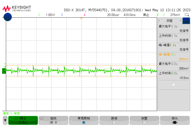
Figure 7, Output ripple & noise ( I_{out} = 30\text{A} )
