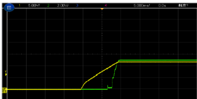
Figure 6, Output voltage established (Iout = 5A)
